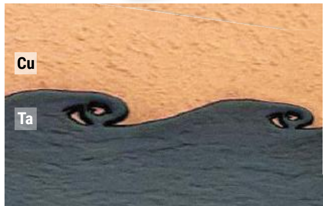
Tantalum - Copper explosive welded interface
