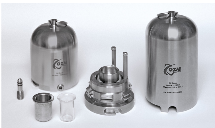
BCA 500 EX and DC bombs for low and high pressure combustion respectively
