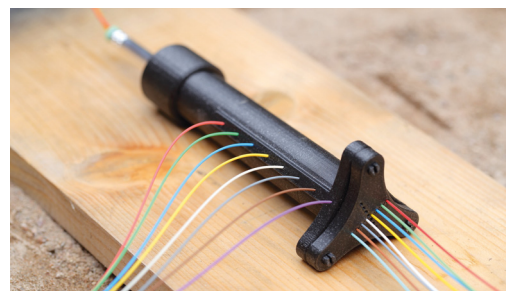
Simultaneous detonation velocity and shock curvature measurement
