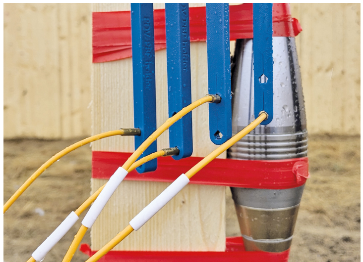
Measurement of the initial velocity of fragments in field tests
