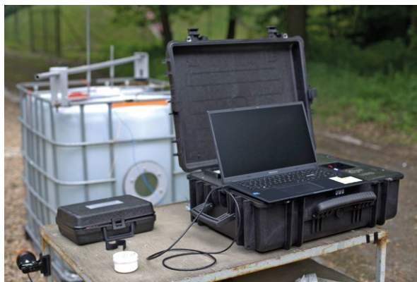
UWB device prepared for detonator test in 1m 3 tank.
