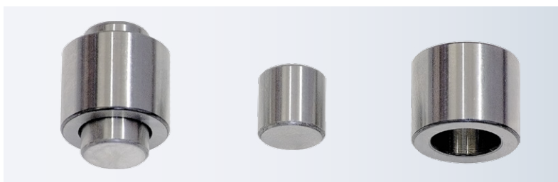
BAM Fall Hammer (Impact Tester) – steel cylinders and guide rings
