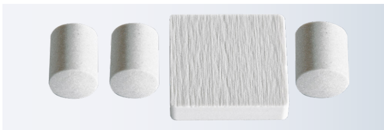
BAM Friction Apparatus – porcelain pegs and a plate
