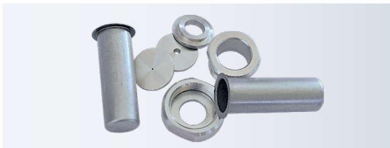
Koenen Steel Shell Tester – test tubes and closing parts
