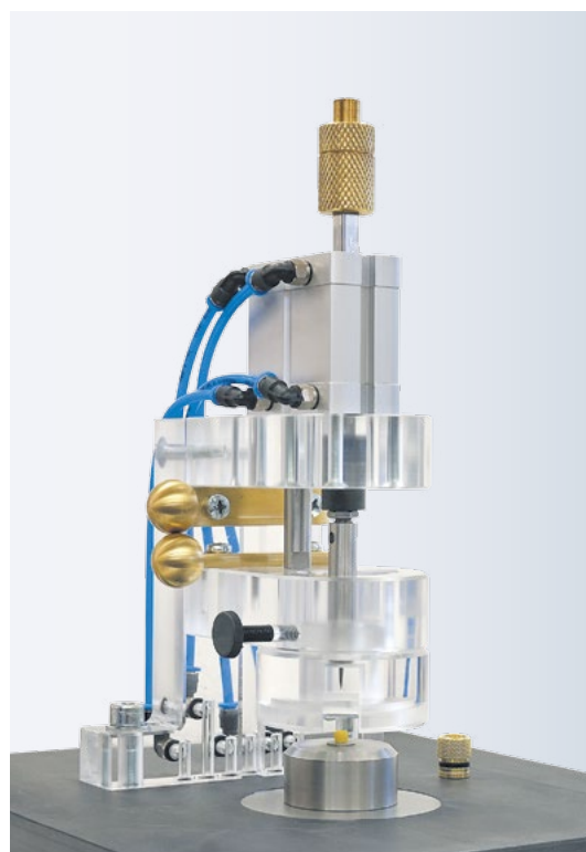
Approaching needle testing stand
