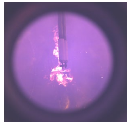
Afterburning of 9.5 % by vol. of methane in air
