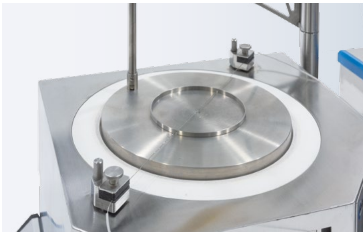
Measurement of temperature uniformity on the hotplate
