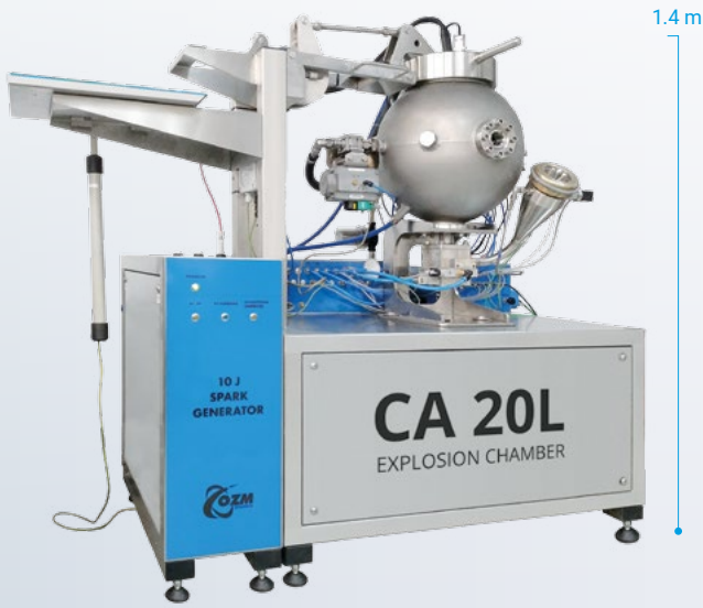
CA 20L explosion chamber
