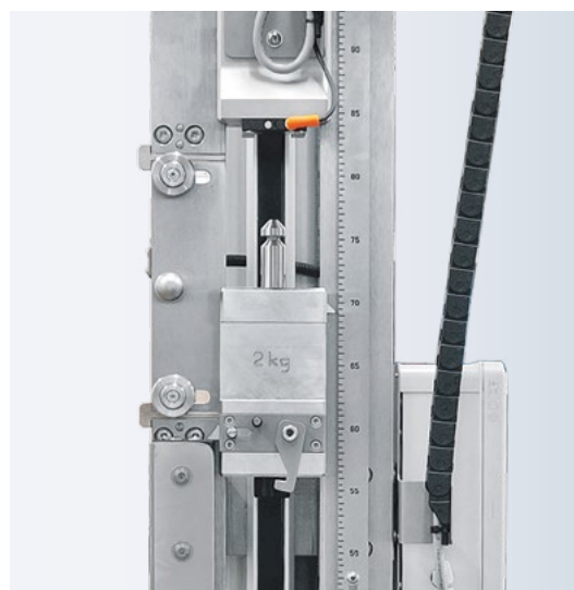
Drop Weight Exchange Window
