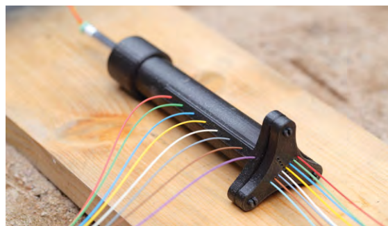
Simultaneous detonation velocity and shock curvature measurement
