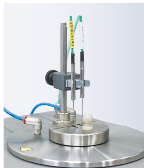
DTA 552-Ex – detail of the furnace
