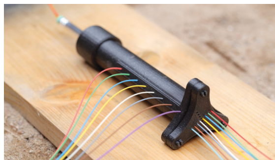
Simultaneous detonation velocity and shock curvature measurement
