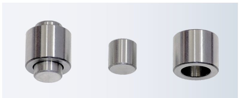
BAM Fall Hammer (Impact Tester) – steel cylinders and guide rings
