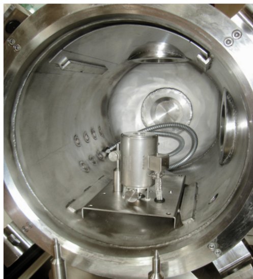
Interior of the container with an electrical heating block
