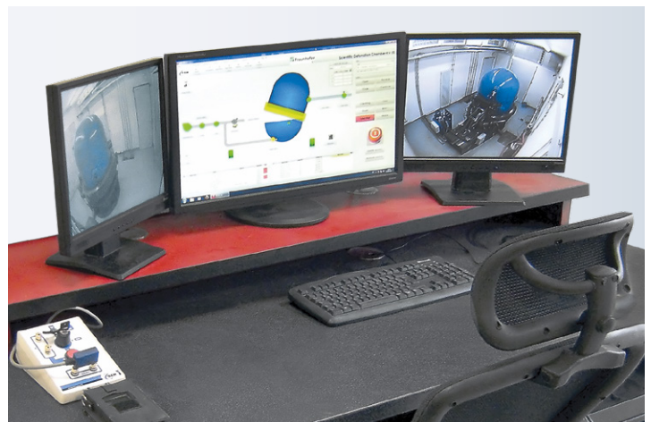
Control panel of the detonation chamber
