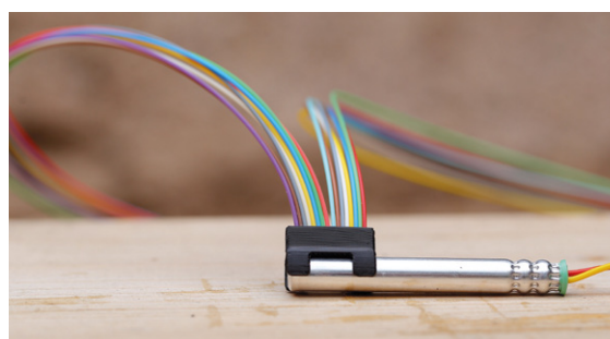
Detonation velocity measurement of a blasting cap
