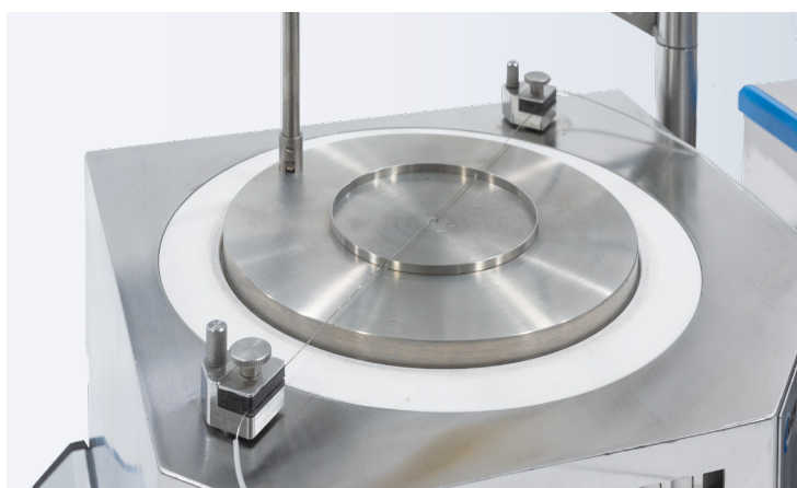
Measurement of temperature uniformity on the hotplate
