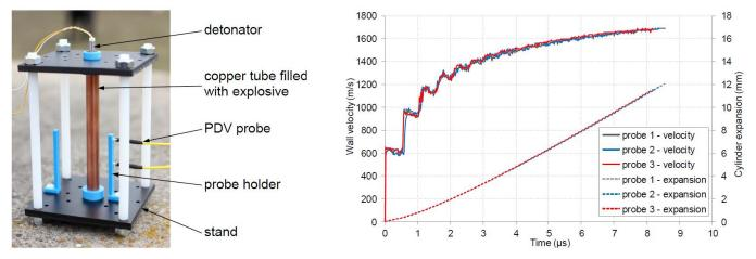
The PDV-DBP probes were used for this small scale <u>experiment with erythritol tetranitrate</u>. In this arrangement, detonation velocity can also be determined simultaneously from the times of arrival of the PDV signals.
