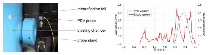
A large blasting chamber was loaded with high explosive charge placed in its center. The PDV-PBP probe allowed to measure velocity of the chamber wall as it was accelerated by shock waves generated by the explosion. Ringing of the wall continued until the end of the recording time window. **Displacement was obtained by integration of the velocity profile** for the most intensive pair of peaks. The maximum displacement agreed well with preliminary numerical model predictions.
