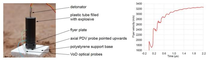
A single PDV-DBP probe was used for the test of sensitized nitromethane (PLX). Additional passive optical probes were employed for simultaneous detonation velocity measurement using OPTIMEX-8 instrument.
