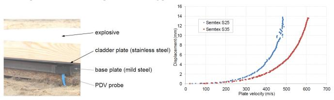
The PDV-DBP probe was fixed in a custom-made probe mount attached to the base plate. The difference between the two types of Semtex S <u>has been revealed</u>.
