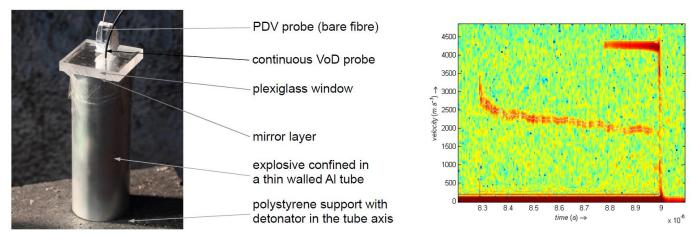
A bare fiber probe was used for this test. Detonation velocity was measured simultaneously using the OPTIMEX-8 with continuous perforated fiber probe inserted in the charge parallel to its axis.
